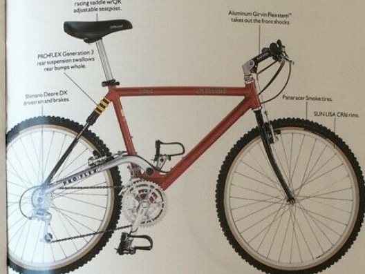
PRO-FLEX 952 FEATURES RIGID CROMOLY FORK & FLEXSTEM XST
