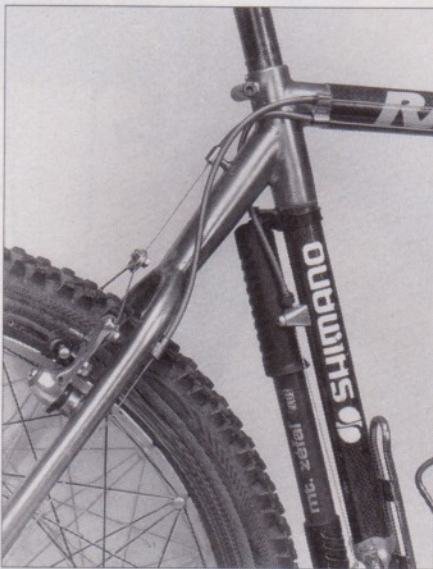
Glued tubes: The carbon fiber frame tubes are joined by titanium lugs made by Merlin Metalworks.
