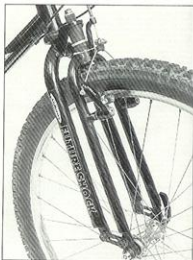
FutureShocks: With a hair over 1" of travel, the FutureShock springer-style forks seem to create overly light steering. We wore out the fork bumpers in less than 100 miles (albeit hard miles).
