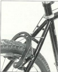
Bolt-ons: Joe Murray must have an aversion to barbecuing his frame designs because the seatpost collar is a slip-on unit and the rear brake cable guide is a clamp-on. Adding to the bolt-on theme, the Kona Explosif Pro comes with a brake booster.
