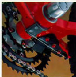
Klein's tradition of innovation includes its patented Chain Control Device ™ , standard on all 1992 mountain bikes. The device keeps the chain from slipping up between the chain ring and chainstay by sweeping it clean and avoiding chain suck.
