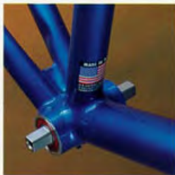
All Klein frames are made in the U.S.A. and offer exclusive design features. The patented chainstay on the drive side has a thicker wall for added stability at the point of greater stress. The bottom bracket is extended and offset to increase power train rigidity, while reducing bearing loads and friction. And the sealed bearings are directly press-fit into the precision-bored bottom bracket, creating a durable, maintenance-free unit.
