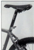
The internal cable routing is about as sleek, sneaky, and to the point as you could ask for. The fillet-style welds are unusual for aluminum, and are extremely nice.
