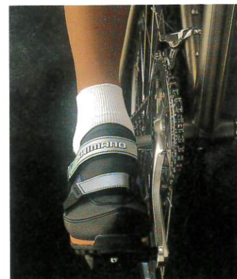
SPD (Shimano Pedaling Dynamics) provides binding pedaling efficiency with a hiking-type shoe.
