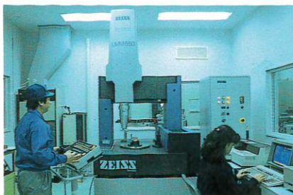
Precise measurements taken with a three-dimensional measuring device.
