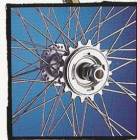
Shredder: Sumo 48 hole alloy rim. Alloy hub. Chrome freewheel.
