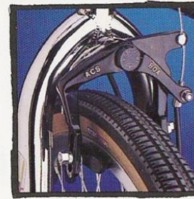
Sport: ACS BOA ball bearing series braking front and rear.
