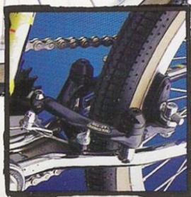
Master: Dia-Compe AD-990 U-braking rear. Haro Multisurface tire.
