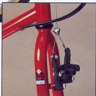
Forks 100% AVR Chromoly. Shimano 201 Cantilever Brakes
