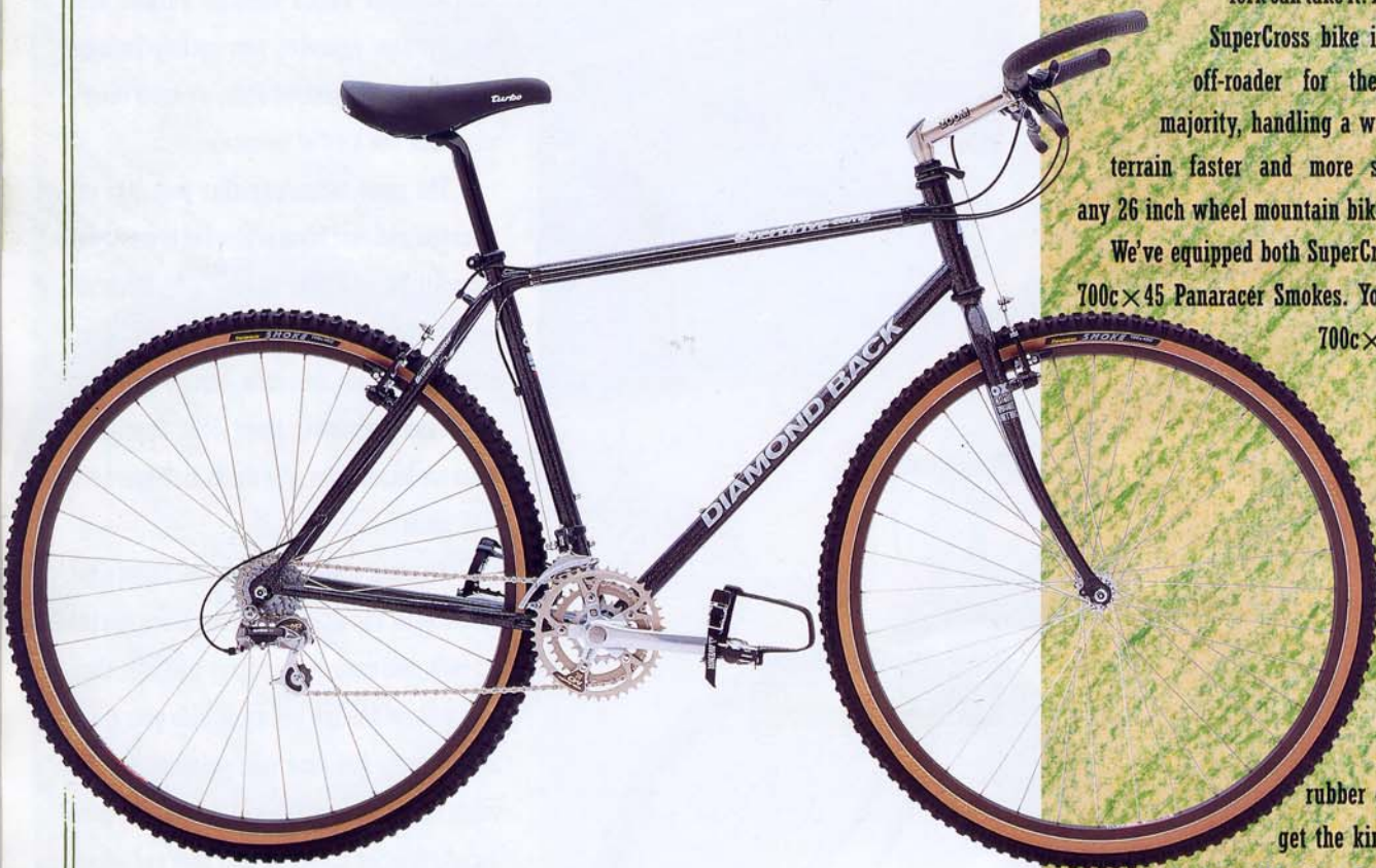
Suntour XC-Pro Micro Drive Crankset 20/32/42T, 11x24T Cassette, and Quick Shifting Short Cage Derailleur
