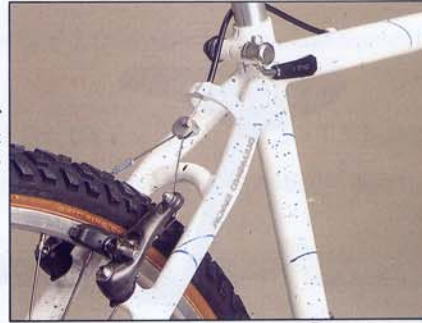
Rear Seat Cluster with Q.R. Seat Post Clamp
