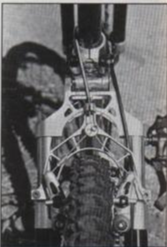
There's a whole lotta air in there! The rear crown is gorgeous, and is stiffer than we thought. The brace won't have windows in final production, though, as a buffer against any excess flex.
