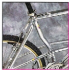
EOS System - Curved seat tube and 403mm elevated chainstays for limitless tire clearance and climbing traction.
