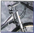
Our rigid upside down triple clamp fork with an Alpinestars braking system provides the front wheel with four inches (100mm) of progressive travel.
