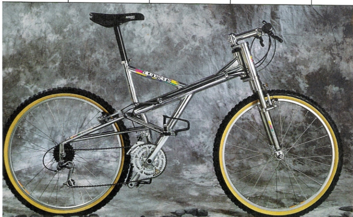
A futuristic frame design that allows a full four inches (100mm) of front and rear shock absorbing travel.
