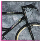
Alpinestars ODS System - 26.6mm 7005 series aluminum handlebars, Easton VariLite aluminum clamp-on stem and Easton VariLite aluminum fork.
