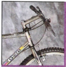
Alpinestars 3-2.5 Titanium oversize stem and Tange Superlite headset.
