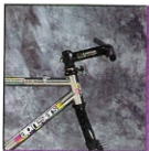
Alpinestars clamp-on stem, Easton VariLite tubing, Tange Superlite headset.
