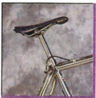
Alpinestars 3-2.5 Titanium seatpost with infinite seat angle adjustment.
