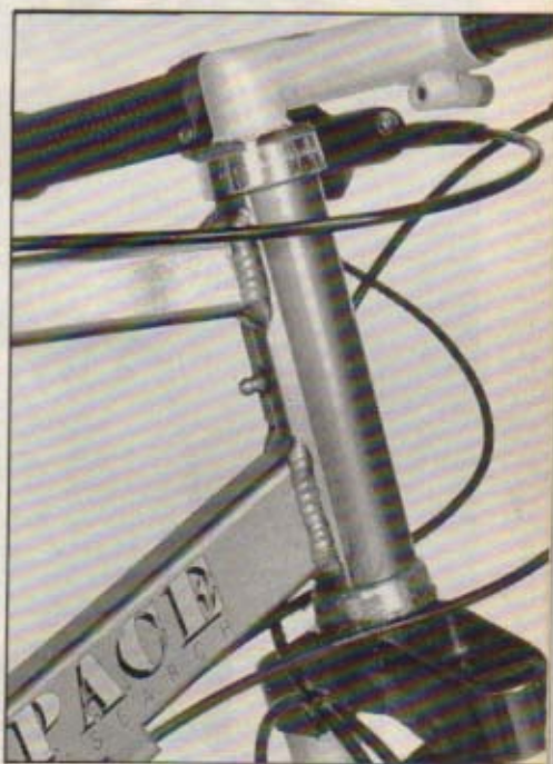
British novelty: The Pace RC-100 sets itself apart from most other bikes in many ways: externally butted square and rectangular alloy tubes, and a trick steering system that requires no headset locknut. The stem and steerer tube are one piece and any adjustment is made by loosening the fork crown.
