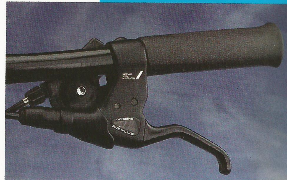
New Shimano Deore XT ST1 Rapid Fire levers with single step-down front shifting and the new Servo Wave brake mechanism for fast cable pick up and improved braking response.
