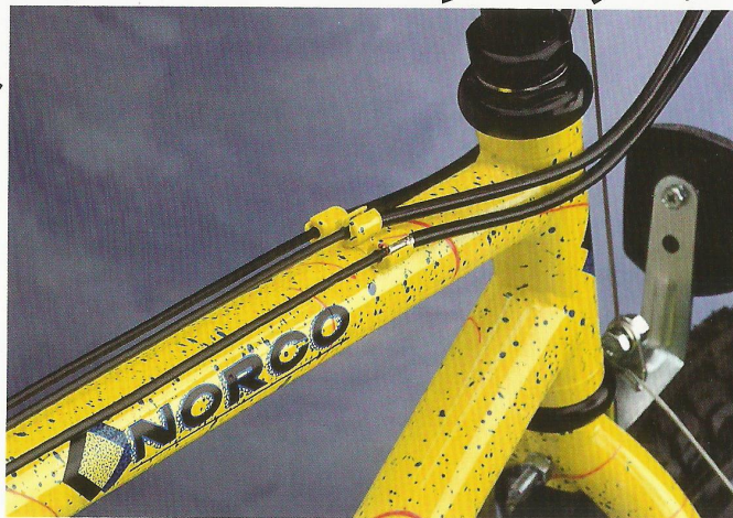
Top-tube mounted open cables reduce friction in the front and rear changer cables and result in increased power to the rear brake by reducing casing compression.
