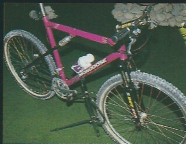
▲ Mongoose's German importer had this half-assembled suspension bike which uses a spring/oil rear shock and a Taiwanese copy of Rock Shox Mk I up front.
