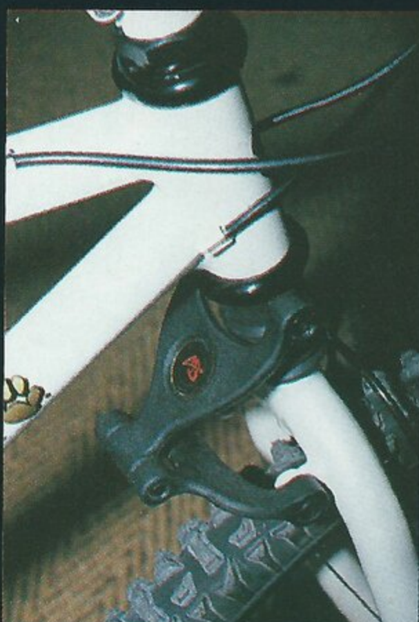
▲ Muddy Fox have joined the growing list of bike makers using the Browning suspension system, which hides the suspension components inside the steerer. Cannondale and Action Tec have superficially similar systems.
