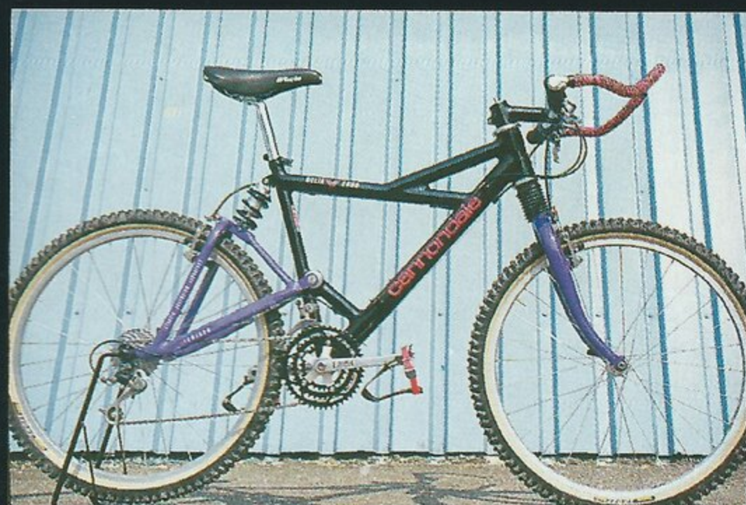
▲ Cannondale's Delta-V is a development of, and improvement on, last year's promising but flawed EST bike. An improved, more rigid rear shock should produce better handling in the back, while the steerer-mounted front suspension is designed to have no lockout so it moves with every bump. Designer Mark Farris reckons a fork should move as much as possible, and after throwing a Delta-V down some gnarly stuff at the Worlds, we agree.
