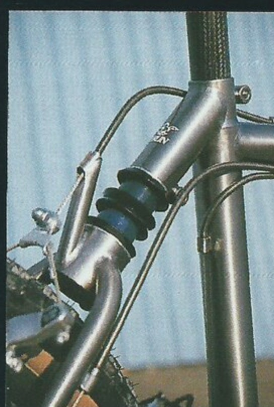
▲ That Merlin suspension bike in detail. The Proflex-style rear shock uses elastomer bumpers but no pivot – the chainstays just flex. Up front the forks move on pivots that project forward from the head tube and the bumper is hidden inside it.
