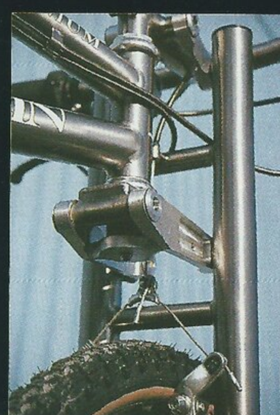
▲ That Merlin suspension bike in detail. The Proflex-style rear shock uses elastomer bumpers but no pivot – the chainstays just flex. Up front the forks move on pivots that project forward from the head tube and the bumper is hidden inside it.
