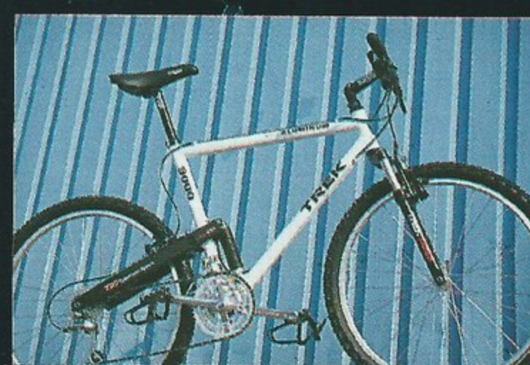
▲ Trek's suspension bike uses an elastomer bumper system in the rear and a gas/oil fork. The fork was developed for Trek by Japanese suspension giants Showa, and is comparable to Rock Shox in weight. The rear unit is all their own work, and provides three inches of travel for one inch of compression.
