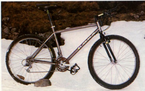
The frame finish is natural titanium, no coating required, as titanium won't rust or corrode why hide it under a layer of paint? The plain finish matched with black Project Two forks, looks really mean and business like - the business being no messin' racin'
