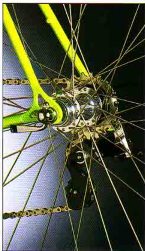
Stainless steel G.P. Wilson dropouts are welded to the stays. Because of the taxing finish work, however, most Slims are using different dropouts.
