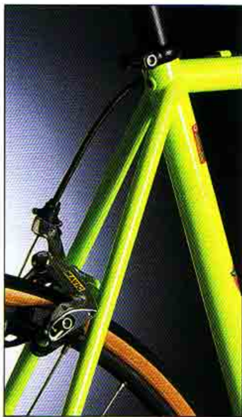
TSX tubing conforms to road-bike tradition. But many more touches (welding, seat collar, split cable guides) hew to Fat City tradition.
