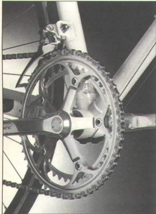
At left: Bottom bracket shell is also cast aluminum; derailleur tab is riveted and bonded.
