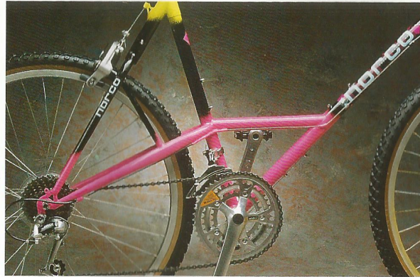
New raised chainstay frame design produces agile handling and eliminates the nuisance of chain suck.
