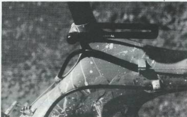
Simply forward mounting the seat post release lets riders quickly adjust saddle height.
