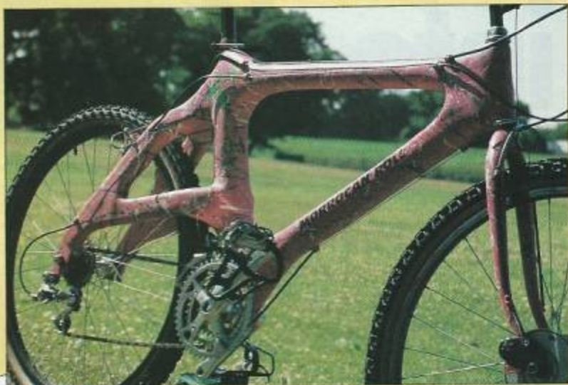
Built for an Industrial Design degree project, The Moroccan Roll features an inexpensive type of composite frame construction
