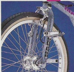
FORKS Featuring screw in hollow fork pegs to prevent bent axles and flip up standers that fold out of the way.
