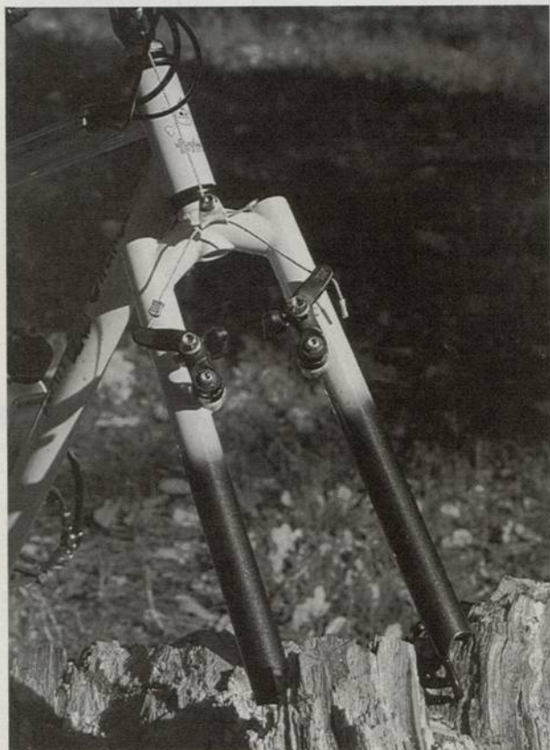
The forks used on the test bike are the forerunner of the upcoming Fat Chance 'Tears of a Crown' forks. Why the pun on the old Smokey Robinson song? Because the fork blades will be ovalized - tear-shaped - at the crown. They will eventually include a rear gusset for maximum strength and weigh in at a very respectable 1lb 12 oz
