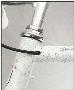
UNIVEGA RUNS THE REAR BRAKE CABLE INSIDE THE FRAME TUBE FOR A CLEANER LOOK. NO CABLE GUIDES TO RUST, BREAK OR SNAG.
