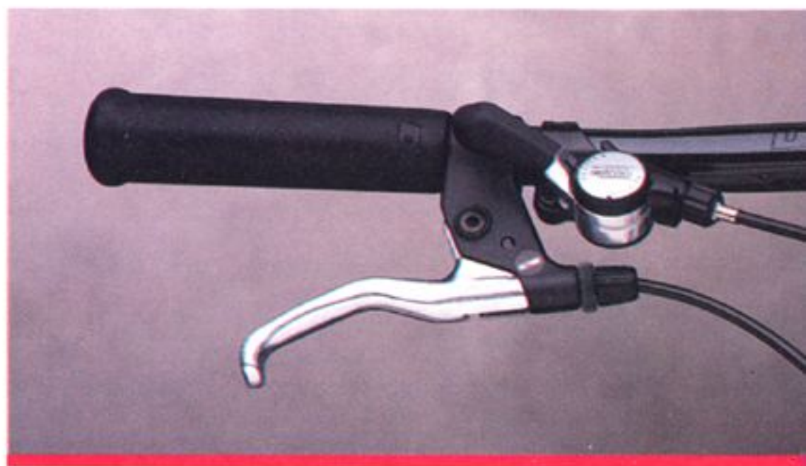
Wrap your fingers around Shimano's ergonomically designed SLR levers for controlled braking power. Adjustable reach, two-finger design.
