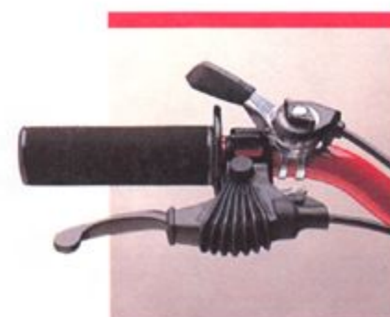
Hooded brake levers are a nice touch and keep out dust and mud.
