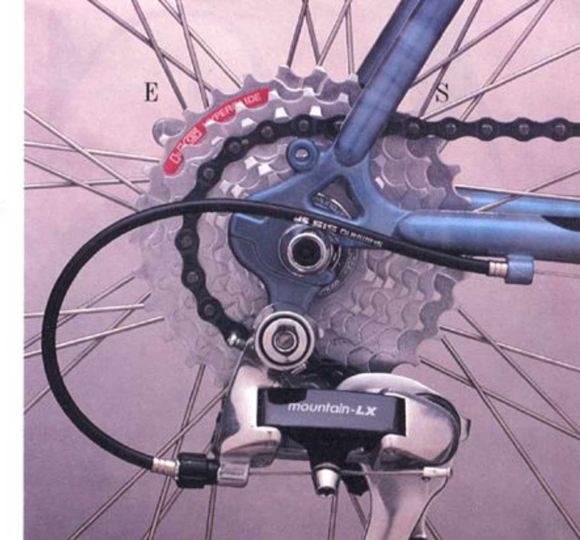
Long cage Shimano Mountain LX rear derailleur and Hyperglide sprockets provide the smoothest, fastest SIS shifting ever.
