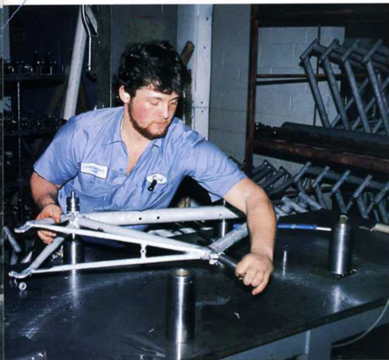
Quality control. Rick Valentine checking frames for proper alignment at our Bedford, Pennsylvania, factory. Photo by Steven C. Wyness
