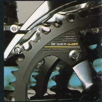
Shimano computer designed Biopace chain rings for greater pedalling efficiency.
