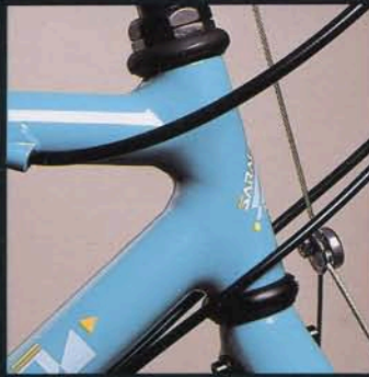
Hand fillet brazing a hallmark of the Kili Flyer and Kili Flyer Competition.
