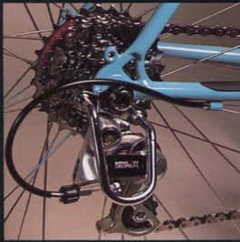
Shimano's new hyperglide 21 speed indexed gear system gives you the ultimate in precise, quick and smooth gear changing even under full pedalling pressure.
