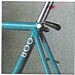
A quick-release seat binder allows you to raise or lower the Viscount Terra saddle for instant adjustment.
