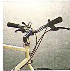
Take control with powerful SLR brake levers and positive thumb-shifters.
