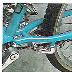
Shimano "U" style brake is mounted onto special braze-ons below the bottom bracket for outstanding braking efficiency.
