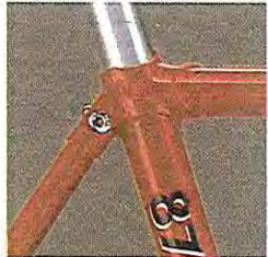
Silver brazing and Trek investment cast lugs make this one of the lightest production chromoly machines in the all-terrain category.
