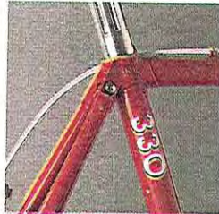
Investment-cast seat lug and True Temper RC-1 tubing combine advanced frame technology and value.
