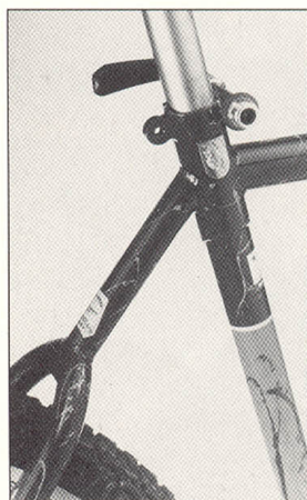
Uni-Stay™ rear end. Note the beefy, investment cast Hite-Rite™ attachment.
