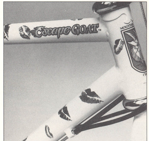
The back of the headtube reinforcing rings are carefully fillet brazed, offering yet another feature that reduces stress at that crucial point.
