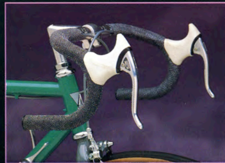
Responsive 105 brake system features Shimano Linear Response levers for excellent response.
