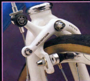
The Weinmann aero levers are coupled to responsive Weinmann 490SQ caliper brakes.
