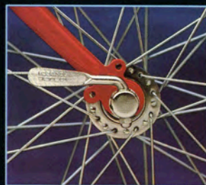
Quick release hub allows convenient no-tool front wheel removal.
