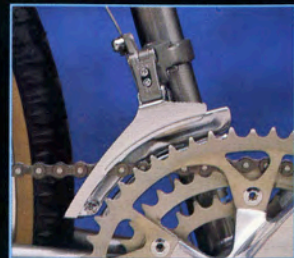
The new Exage Mountain front derailleur features SIS indexing or friction control shifting.
