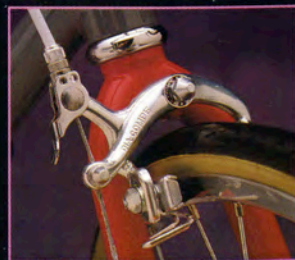
The 3000 features responsive Dia Compe QS400N side pull brakes and AC-260 aero brake levers.
