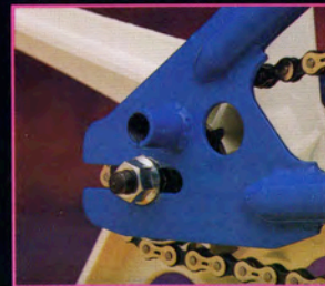
The Stylist has rear threaded bosses for optional foot pegs.
