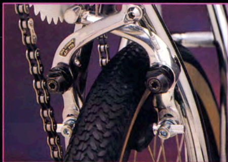
The Dia Compe "U" style brake is positioned on the chainstay, out of the way.
