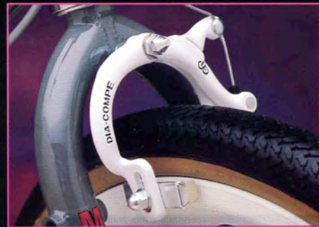
The front Dia Compe brake features a recessed rear nut and quick release feature.
