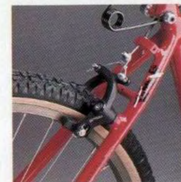
Shimano Deore XT U-brake.
