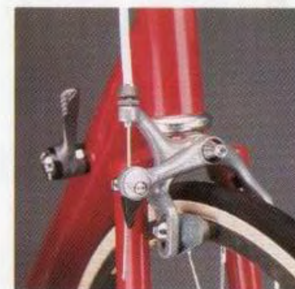
New Shimano 600 Ultegra brakes.
