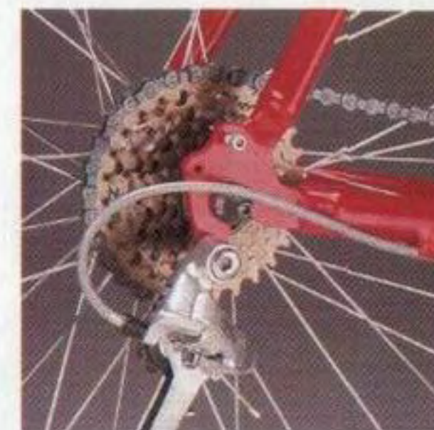
Shimano Deore SIS shifting.
