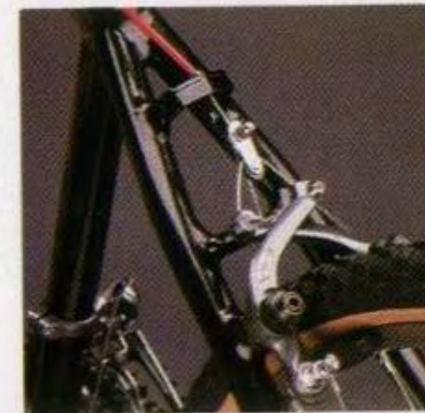
Dia-Compe Advantage brakes.
