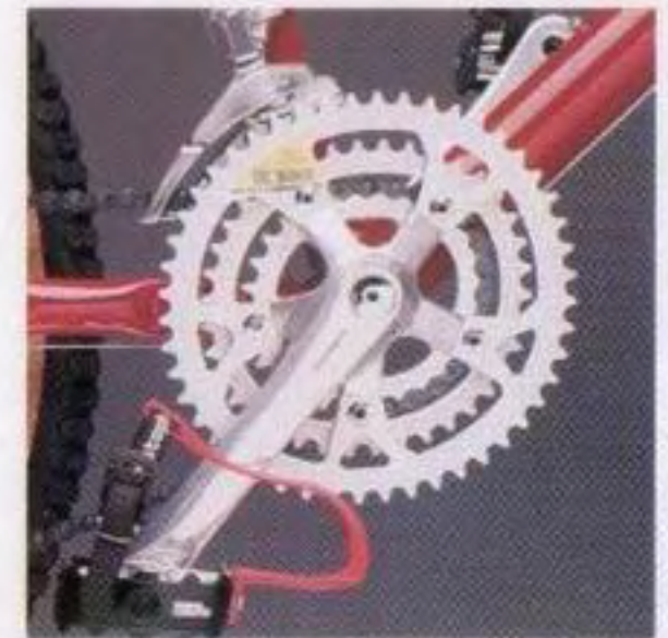
Shimano Biopace crankset and Deore pedals.
