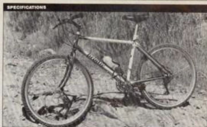
A touch of class: Builder Paul Brodie's attention to detail is flawless on the Romax. The reinforced seat lug and collar guarantee strength and durability.
