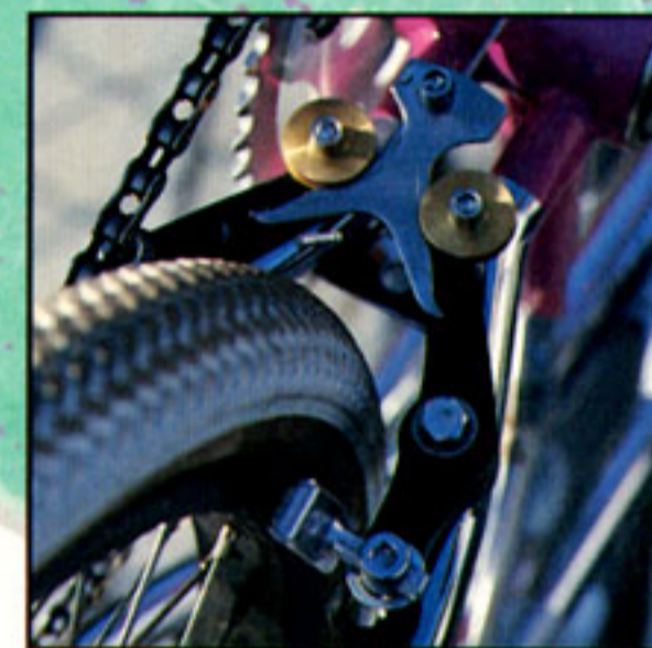
Suntour XC Sport Cam brake gives you better stopping power.
