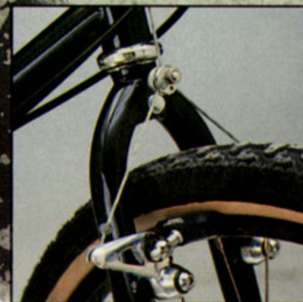
Aero Unicrown fork and 72 degree racing geometry mean quick handling.
