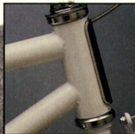
Heliarc welded 1 1/8" tubular chromoly means lightweight durability.
