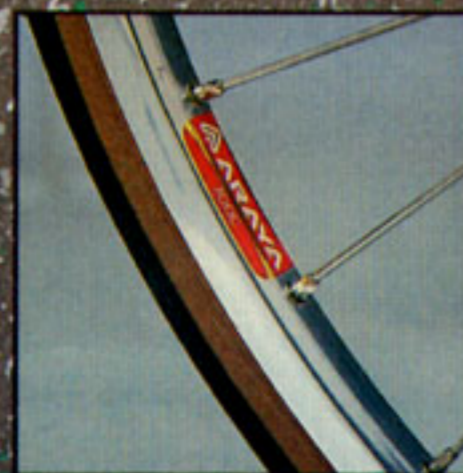
Araya 32 spoke alloy rim laced with stainless spokes.
