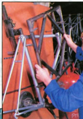
SETTING THE FRAME
