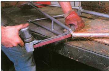
HANDFINISHING THE FRAME
