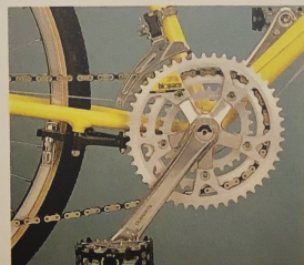
State of the art Suntour XC Sport brake mounted under chainstays. Shimano's unique Biopace crank set offers more efficient pedaling.
