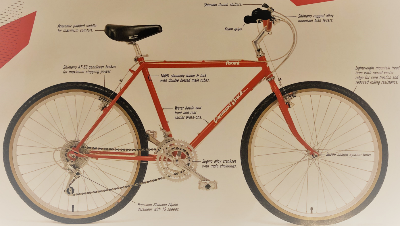
Shimano cantilever mountain brakes offer smooth gradual or instant stopping power.
