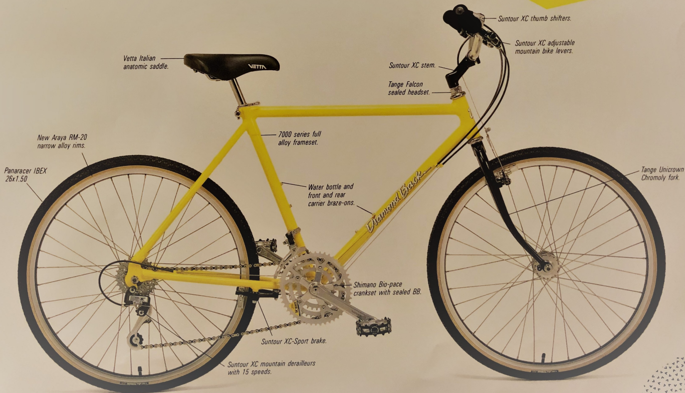
State of the art Suntour XC Sport brake mounted under chainstays. Shimano's unique Biopace crank set offers more efficient pedaling.
