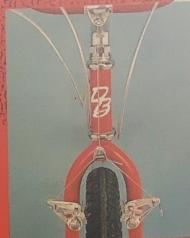
Shimano cantilever mountain brakes offer smooth gradual or instant stopping power.
