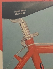
Instantly adjustable quick release seat pillar bolt.
