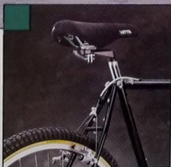
Chromoly tapered direct seat stays with dual quick-release saddle adjustment.
