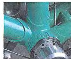
Close tolerance investment-cast bottom bracket shell.
