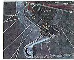
Wide capacity double-articulated Duopar derailleur.
