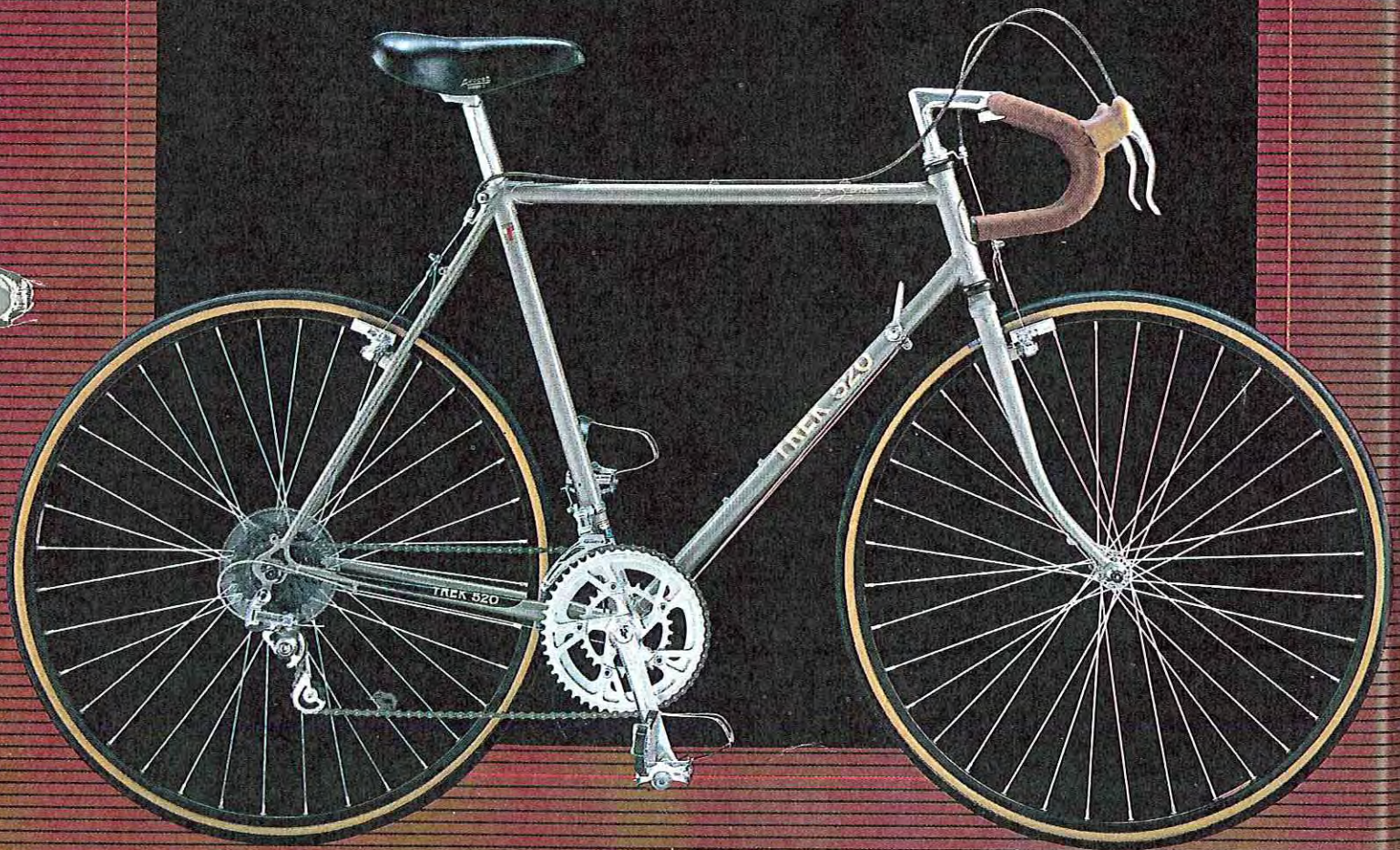
SR's new triple crankset offers 18 well-spaced gears.
