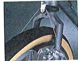
Dia Compe cantilever brakes with motorcycle-type levers.
