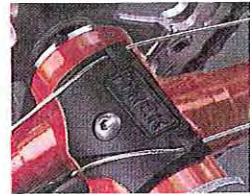
Derailleur cables are routed through a low-friction guide.
