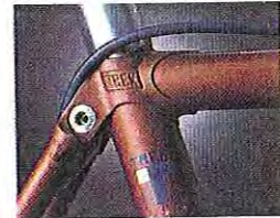
Reynolds 753 tubes joined by Trek's unique cast seat lug.
