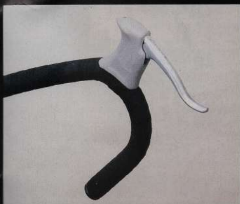
Shimano Adamas hooded levers with concealed cables
