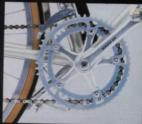
Sugino GS long arm fully detachable chainwheel
