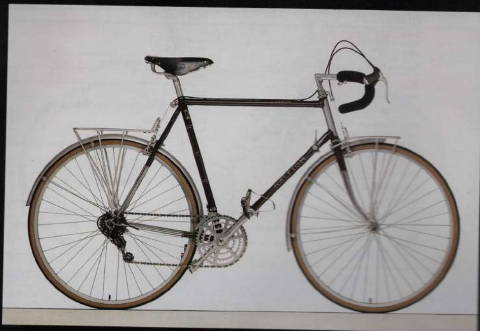
Huret titanium-bodied Duopar gear
