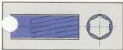
Spiral Stem Reinforced spiral ribbing to strengthen critical stress areas of the stem.
