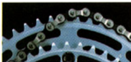
Gear shift on W-cut Teeth
