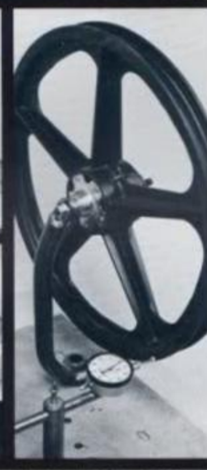
Final Quality Control: Parts are checked on a frequent basis for concentricity and appearance.
