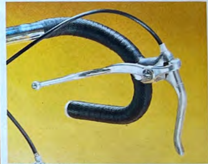
Brake Levers Operate two ways, GT extension levers having been fitted. Perfect brake control for "on-top" riding.
