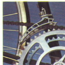
2 - Alloy Cotterless TA double chain-wheel and cranks.
