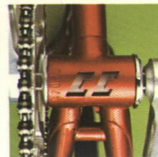
2 - Carlton initial cutout in bottom bracket shell.
