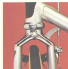
2 - Forged integral sloping fork crown.
