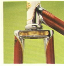
3 - Front fork blade stiffeners.
